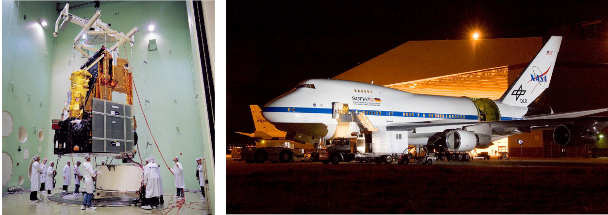
Figure 2: L: the INTEGRAL space telescope, with people for scale. This photo was taken in 2002 while INTEGRAL's Flight Module being prepared in ESTEC's facilities in Noordwijk, the Netherlands. INTEGRAL is a gamma-ray telescope. Image credit: ESA - A. Van Der Geest R: the Stratospheric Observatory for Infrared Astronomy (SOFIA) telescope. The telescope is mounted in the back of a Boeing 747. Flying high above most of the water vapour in the atmosphere enables SOFIA to observe IR radiation.
