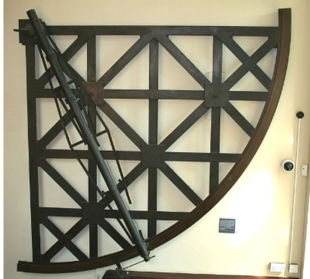
Figure 7: A wall-mounted mural quadrant. Until atomic clocks were commonplace, the use of a quadrant to time transits of stars across the meridian was the most accurate method of timekeeping.
