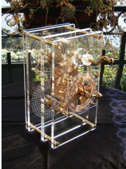
Figure 8: A 2007 reproduction of the Antikythera mechanism, an ancient device for predicting eclipses and other astronomical events.
